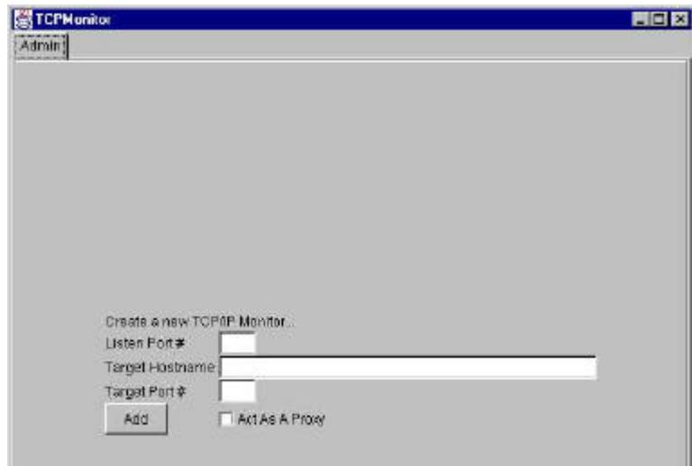
To use the program, you should select a local port which `tcpmon` will monitor for incoming connections, a target host where it will forward such connections, and the port number on the target machine which should be "tunneled" to. Then click "add". You should then notice another tab appearing in the window for your new tunneled connection. Looking at that panel, you'll see something like this:
